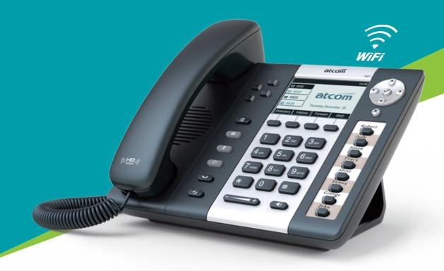
A41/A41W is a 4 SIP accounts, multiple features, easy deployment, and Wi-Fi optional IP Phone, which has 3.2-inch FSTN 4 level grey LCD, 4 soft keys, 8-speed dial programmable keys extending to 88 keys, convenient operation performance, and TIA920 high definition wideband voice standard, with clear HD voice. It is designed for business level enterprise unified communication application.
