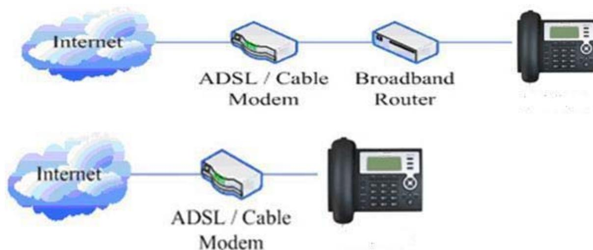
Shared network connection—Use this method if you have a single Ethernet port in your workspace with your desktop computer already connected to it. First, disconnect the Ethernet cable from the computer and attach it to the WAN port on the back of your phone. Next, use the Ethernet cable in the package to connect LAN port on the back of your phone to your desktop computer. Your IP Phone now shares a network connection with your computer. The following figure is for your reference.
