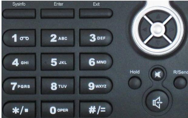
The numeric keypad with the keys 0 to 9, \*, and # is used to enter
